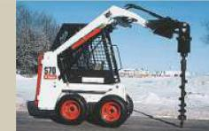
Auger Drills holes with speed and plumb-line accuracy.
