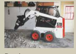
Breaker Breaks up concrete and asphalt quickly and effortlessly.
