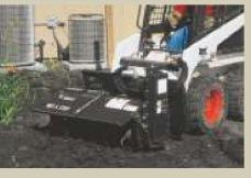
Tiller Digs and loosens soil; mixes compost and other materials into existing soil.
