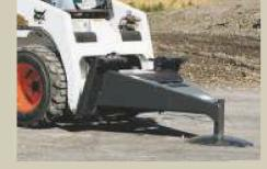
Mini Scraper Cleans ice and snow off parking lots; scrapes floors; removes tile flooring.
