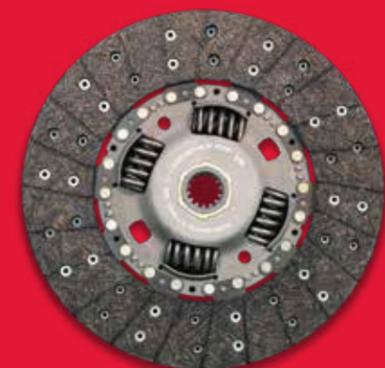
Both the FURIO 7 HD and the FURIO 7 Tipper come with an LUK Clutch; of 280 mm and 310 mm diameters respectively. The bigger diameter provides more contact area and better power transmission without any slippage. There's even a booster to lower the effort of clutch operation and higher lining life to lower maintenance cost. What's more, there's a wear-indicator to let you know when you need to replace it.
